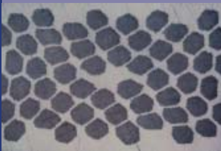
From Tore Supra superconductors R&D: NbTi strands (10 000 filaments – 23 microns diam.), large-scale fabrication (20 tonnes in 1984-86) with continuous control.
