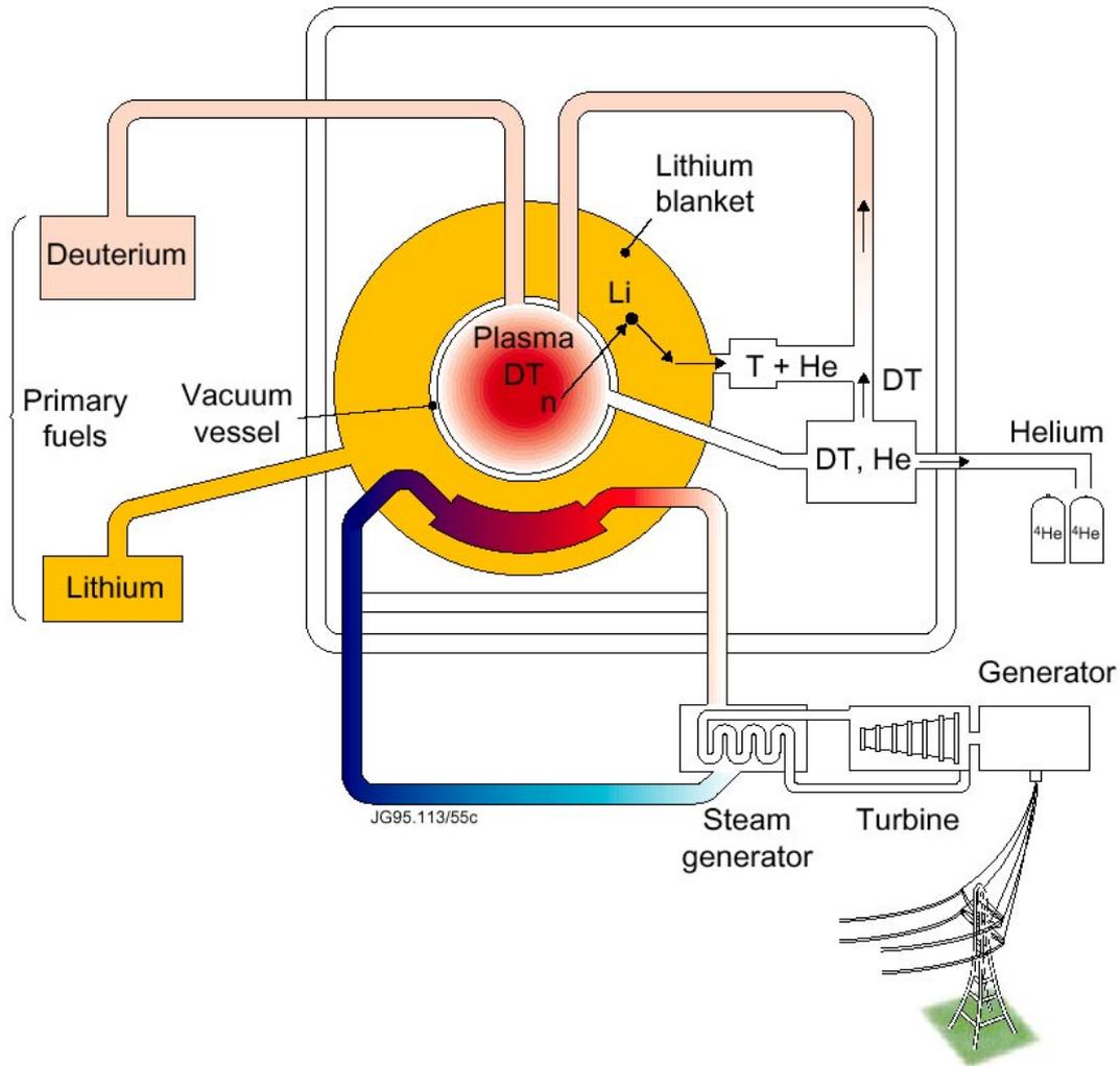
Figure 1: Schematic diagram of a fusion power station
