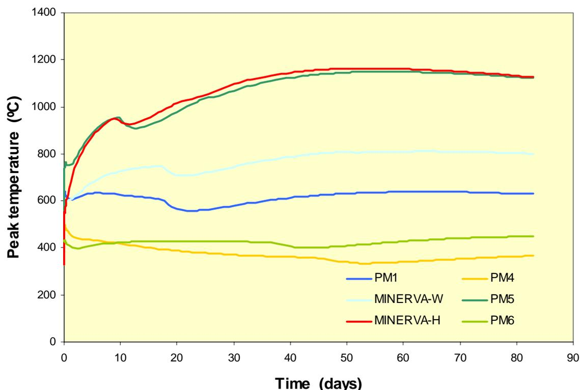
Figure 9: Conservatively calculated peak temperatures following hypothesised loss of all coolant, and no credit taken for any safety system or mitigative action, for the six SEAFP designs.
