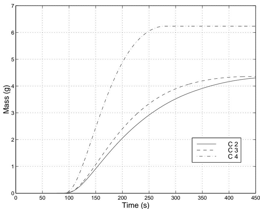
Figure 10: Calculated releases of dust to the environment for an accident in MINERVA-W, with Type C containment system
