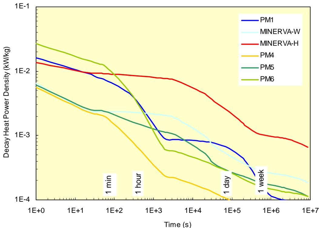
Figure 5: Decay heat power density, averaged over the blanket, for the six SEAFP blankets.
