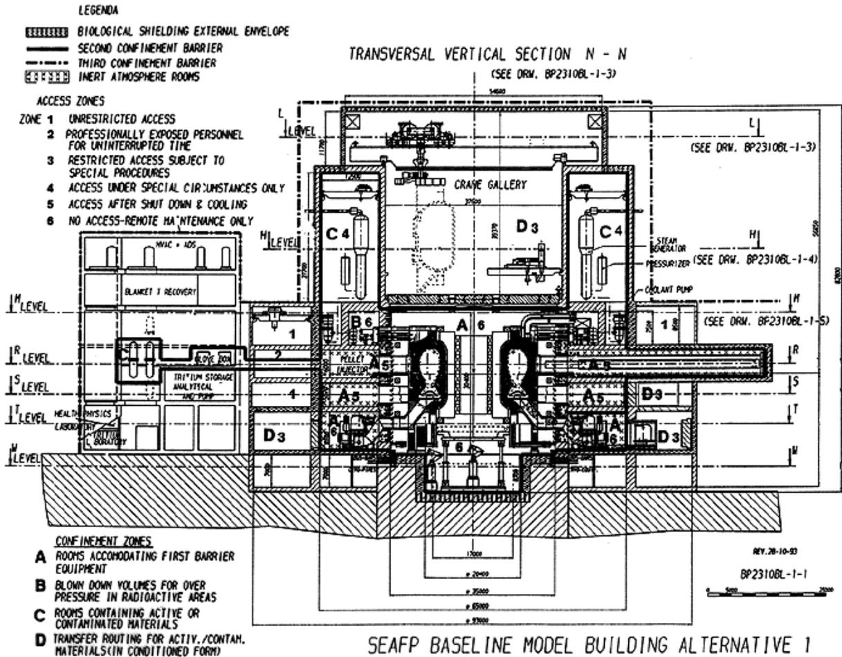
Figure 3: Vertical section of the core, surrounding buildings, and tritium plant of the designs of fusion power stations considered in these studies
