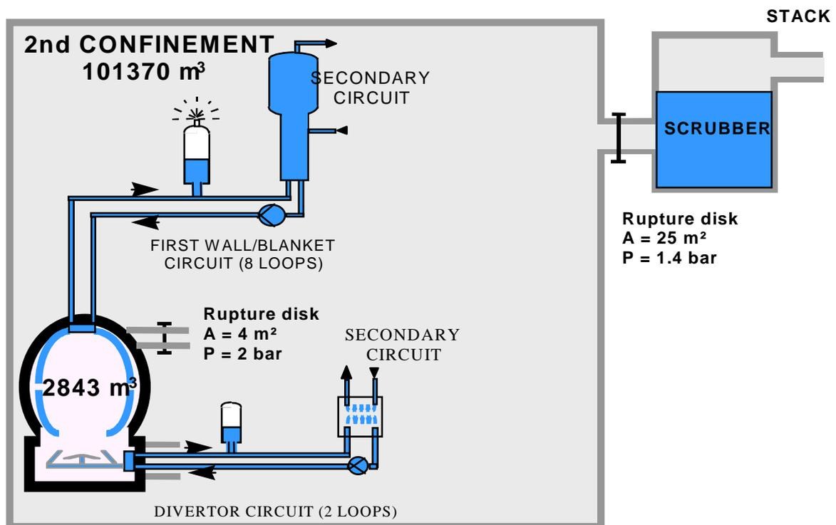
Figure 4: Schematic diagram of a containment system
