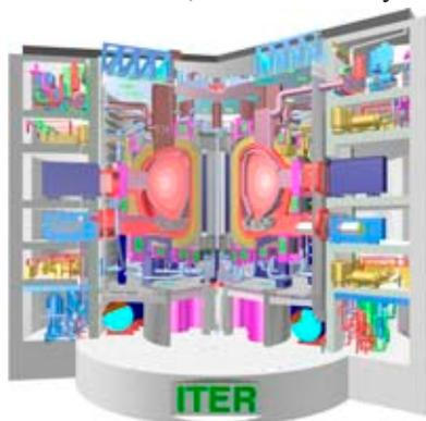
**Cut-away model of the International Thermonuclear Experimental Reactor (ITER) with 6.2 m radius and a projected fusion power of 500 MW. Inside the D-shaped superconducting coils the vertically elongated plasma doughnut can be seen.**
