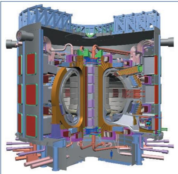
*Cutaway view of the ITER reactor*
