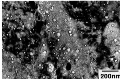
*Micrograph showing an example of material swelling under irradiation. Voids have been formed in a low activation steel (F82H) leading to 1% swelling.*
