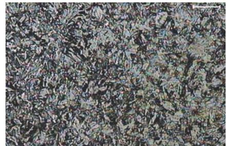
*Magnified images of the microstructure are a common working tool for material scientists to investigate their material samples, in this case of EUROFER 97.*
