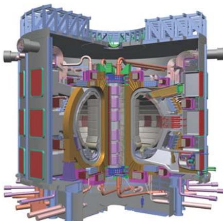
*A cut-away drawing of the ITER tokamak, showing the D-shaped vacuum vessel surrounding structures, and the 24 m high cylindrical cryostat, which forms one of the safety barriers.*
